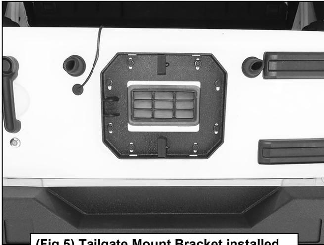
(Fig 5) Tailgate Mount Bracket installed
